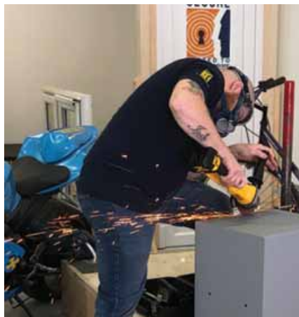
Just to show what's involved in the Gold Level test Guy demonstrated an angle grinder attack - as it happens the double skinned Mini Vault Gold FR may well have passed this particular part of the higher level test
