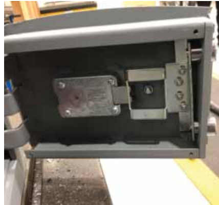
This picture shows how the boltwork had distorted when being forced back and defeated Guy's attack
