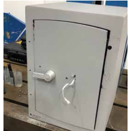
The double skinned Mini Vault FR safe after Guy had finished his attacks. The door would still open!
