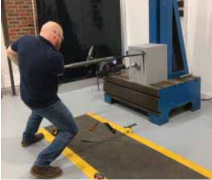
Adding some extension pieces increases the force dramatically
