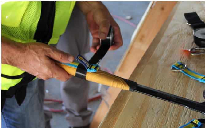
ToolMate® Link Strap Attachment with D-ring (RTM-LS2.25) used with Attachment Tape
