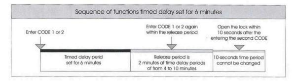
Activate timed delay (only with the electronic lock open):
