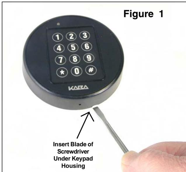
To replace the battery, you must first remove the keypad assembly.
