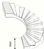
4. 180 degree circular staircase
