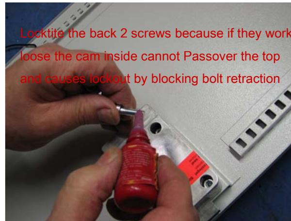
Locktite the back 2 screws because if they work loose the cam inside cannot Passover the top and causes lockout by blocking bolt retraction
